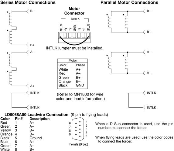
Use twisted pairs, shield open at backshell.
